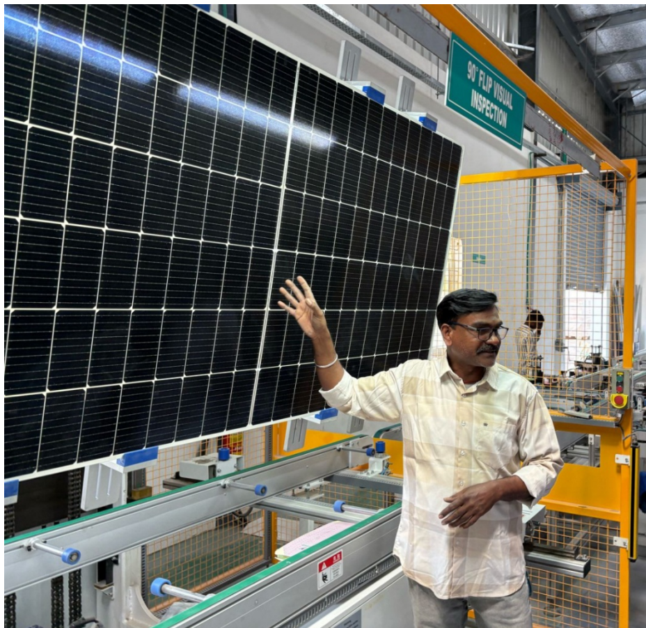
3. 90 Degree Flip Visual Inspection
